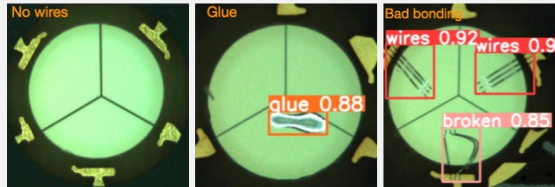
Figure 5- Images from wire bond holes annotated using Roboflow platform for object detection. The object of interest is enclosed in the bounding box and given a label name such as glue, wires, or broken wires.
